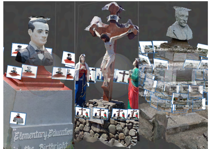
Figure 7. The Photogrammetric Reconstruction Process of the Statues
